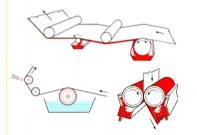
Several application methods for the surface treatments using this technology
